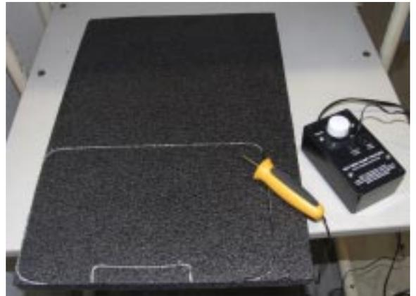
3) When melted foam builds up on the Hot Knife blade it can be cleaned by gently wiping it while it is switched on and fully heated against a paper or cloth towel. Never pinch and tug at the blade as this could pull it from its mount.
