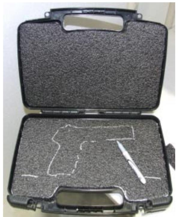
7) Shape the blade of the Freehand Router to fit between the lines traced onto the foam. Carefully carve the foam to the desired depth. Cut just deep enough of a cavity for the equipment to snug firmly against the top foam piece when the case is closed.
