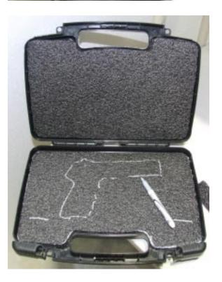
7) Shape the blade of the Freehand Router to fit between the lines traced onto the foam. Carefully carve the foam to the desired depth. Cut just deep enough of a cavity for the equipment to snug firmly against the top foam piece when the case is closed.
