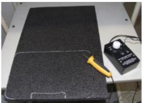
4) Cut out the Armor Foam for the top of the case. In this case, it will be identical to the bottom insert.
