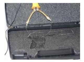
8) All that were needed to hold the two magazines in place were slits. Double check to make sure that your gun or other instruments and accessories fit snuggly in the cutout. You want as tight a fit as you can get without it being too difficult to close the case.
